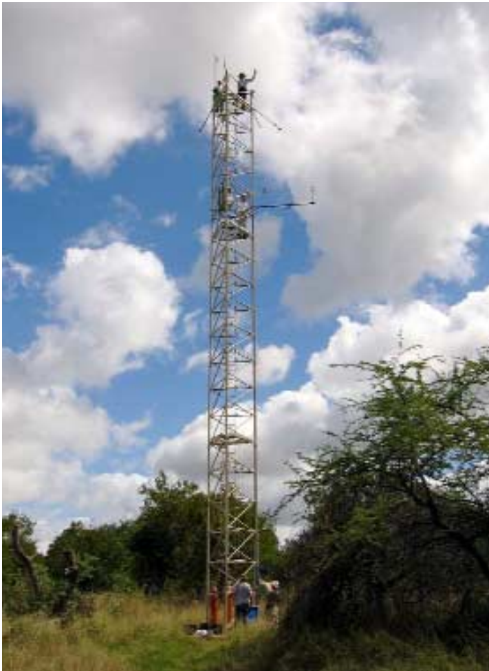
This tower is an experimental setup for meteorological measurements of CO 2 exchange by a savanna ecosystem in Kruger Park, South Africa.
