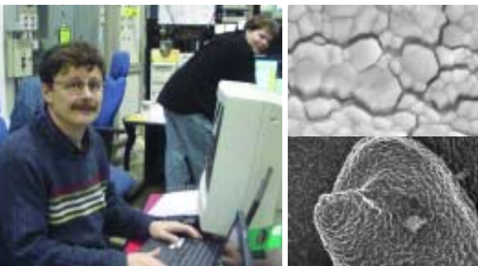
Alexander Goncharov (left) and a colleague conduct research at the HPCAT Beamline. Crystals of iridium nitride (top right) and of platinum nitride (bottom right) are visible in this pair of scanning electron microscope (SEM) images.
