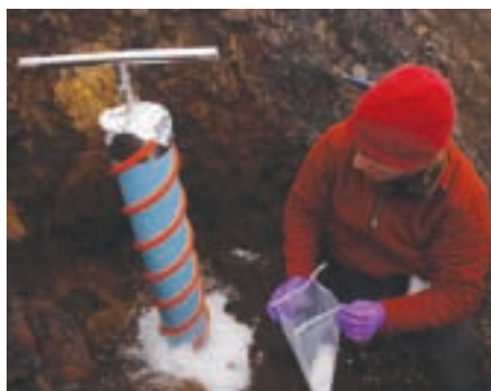
GL's Andrew Steele examines an ice-coring tool penetrating blue ice.
