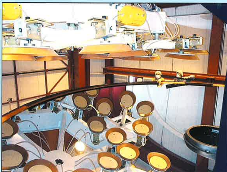
The Walter Baade telescope mirror was coated with aluminum for the first time on August 7, 2000. It has an average reflectivity of 90%—an excellent achievement. The lifting fixture is shown above and reflecting in the mirror.
