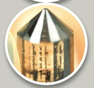
This colorless diamond (top) was cut from a 1-carat block created by the Geophysical Laboratory's diamond-making team using its unique chemical vapor deposition (CVD) process.
