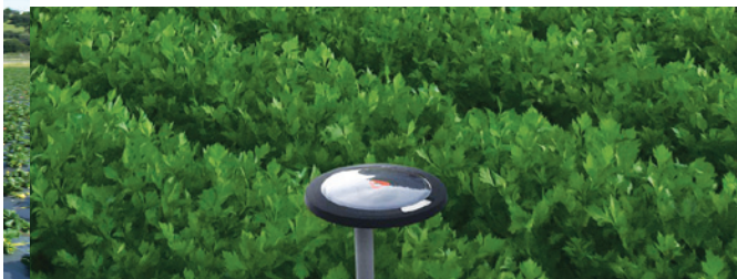
Adam Wolf (right, in photo at left) is in a field in Salinas, California, with the first-of-its kind Pulsepod, produced by Arable, a company that he cofounded. The 6½-inch diameter, solar-powered tool (above) measures rainfall, water demand and water stress, microclimate, canopy biomass, light-use efficiency, and more.
