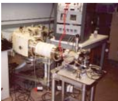
Research in cosmochemistry requires determining the atomic species, or isotopes, of minute quantities of material found in meteorites. The electrostatic analyzer, which Louis Brown has worked on, is being tested for use with the ion microprobe.
