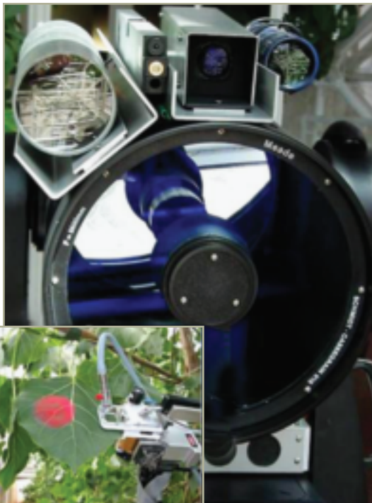
Fig. 2. This prototype remote sensing instrument for chlorophyll fluorescence operates at distances of up to 50 meters from the target leaf or canopy. The insert at lower left shows a target leaf being illuminated by the laser. The equipment attached to the leaf permits simultaneous measurements of photosynthesis and fluorescence for calibration. (Image courtesy Barry Osmond.)
