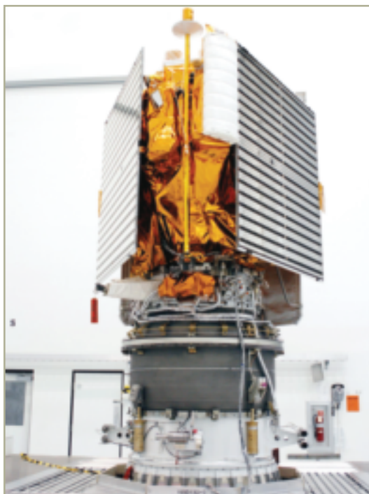
Fig. 6. The complex process of assembling and testing the MESSENGER spacecraft and mating it to its launch vehicle extended over a year and a half. Shown is the spacecraft on July 14, 2004, after it was attached to the payload assist module of the Delta II third stage at Astrotech Space Operations in Titusville, Florida. The two flat, reflective panels are the solar arrays stowed in their launch positions. (Image courtesy NASA and The Johns Hopkins University Applied Physics Laboratory.)
