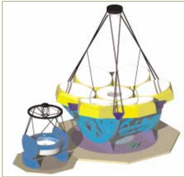
Fig. 2. The current design of the Giant Magellan Telescope (GMT) is shown side by side with one of the Magellan 6.5-meter telescopes. The two human figures by the GMT are shown for scale. The GMT will revolutionize our knowledge of nearby planets and provide a window on the earliest moments of our universe.
