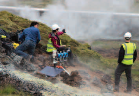
17 From left to right: Alberto Behar, Linda Elkins-Tanton, and James Tanton are on a fumarole in Iceland with a BENTO box, which measures volcanic gases and weather conditions.
