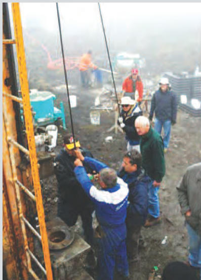
15 The DTM team installs a strainmeter near the Etna volcano.
