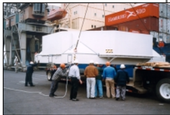
In Coquimbo, Matt Johns (white jacket) and Peter de Jonge (brown jacket) monitor the placement of the mirror on a rare air-ride trailer.
